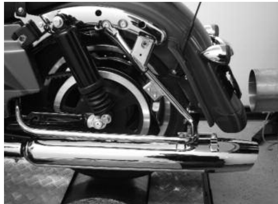
2 Rob starts by using a 9/16" deep socket to remove the stock muffler clamp.
