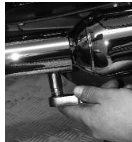
2 Rob starts by using a 9/16" deep socket to remove the stock muffler clamp.
