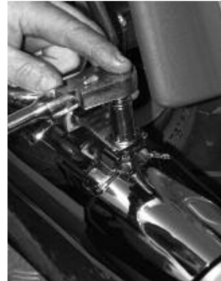
3 He uses a 1/2" socket to remove both muffler support bolts.
