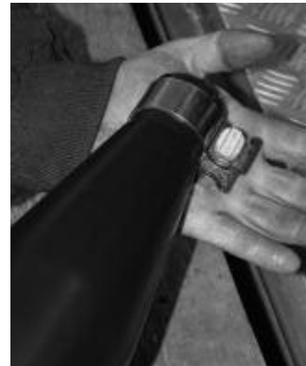
5 He moves the stock clamp from the stock muffler to the new Von Braun Radio Flyer muffler and slips the muffler onto the stock pipe.
