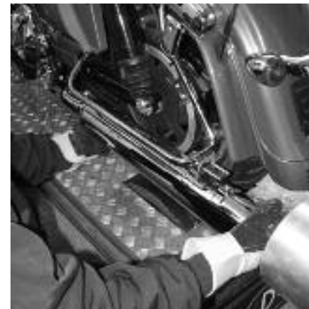
4 Rob pulls the stock muffler from its pipe. He has to gently wiggle it from side to side to get it to come loose.
